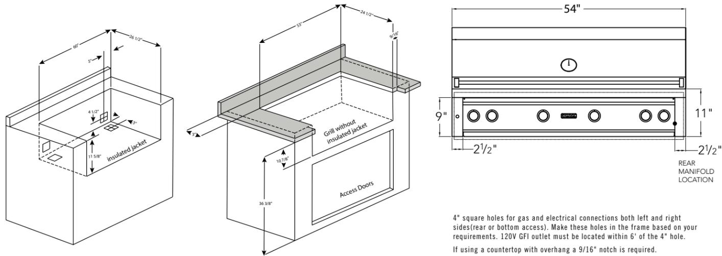
4" square holes for gas and electrical connections both left and right sides(rear or bottom access). Make these holes in the frame based on your requirements. 120V GFI outlet must be located within 6' of the 4" hole.
