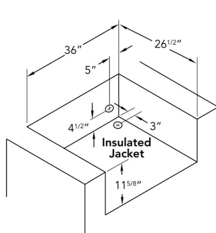
4" square holes for gas and electrical connections both left and right sides (rear or bottom access). Make these holes in the frame based on your requirements. 120V GFI outlet must be located within 6" of the 4" hole.
